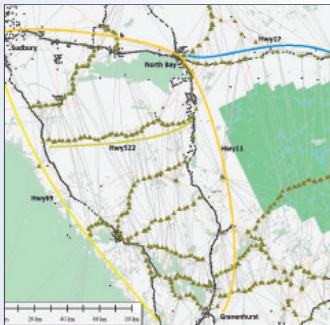
Figure 1. Map showing part of the Ontario Control Survey System. The Black dots are control points in NAD83 (Original) only. The brown triangle points have been surveyed in both NAD83 (Original) and NAD83 (CSRS).
